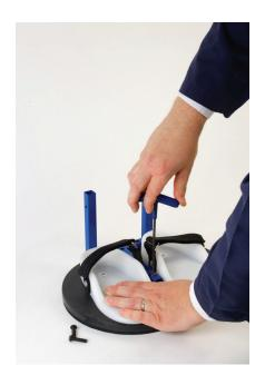
Insert the side struts (D) into the two vertical tubes of the base bracket. Secure with the #10-32 machine screws and self-locking nuts in the uppermost hole of the three holes provided. This allows for growth adjustments later.
