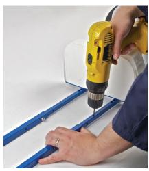
Refer to the measurement sheet and obtain the floor-to-gluteus maximus measurement. With the center of the gluteal panel corresponding to this height, drill one hole on the front face of each side strut to allow for the attachment of the gluteal panel. Align gluteal panel such that center of panel pre-drilled holes corresponds to gluteal to floor measurement holes. Mark height on side struts and drill through front face with 3/16 in. bit. Secure the parts using the 3/16 in. pop rivets.
