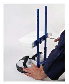
Insert the upper ends of the side struts into the back support. Using the upper most hole as a reference, slide the back support up and down until the top hole corresponds with the axilla-to-floor value on the measurement sheet. When this is accomplished, secure the two pieces together using the #10-32 machine screws and self-locking nuts in the two lower holes provided.
